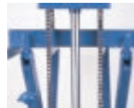
Twin heavy duty lifting chains provide a 2:1 lifting ratio for shorter lift stroke and reduced cylinder wear.
