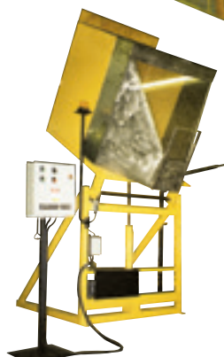
FULLY AUTOMATED DUMPER WITH MANUAL OVER RIDE AND "E" STOP
