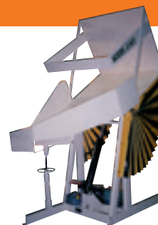
STATIONARY DUMPER WITH ADJUSTABLE CHUTE ATTACHMENT AND SAFETY SKIRTING
